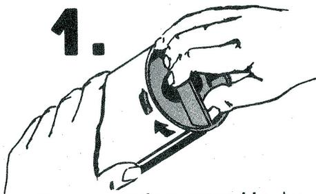
Remove spring assembly by rotating plastic base clockwise until tabs are released from window. Pull bottom out carefully.
