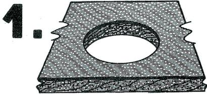
Cut hole size for desired dispenser. To determine proper hole diameter refer to specifications.
