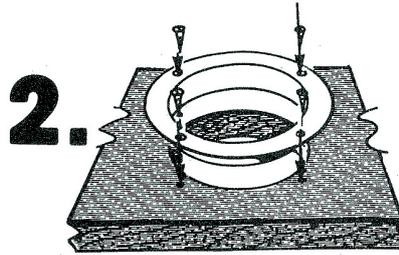
Fasten mounting ring securely over hole with the supplied mounting hardware.
