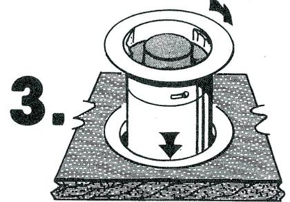
Place dispenser into hole. Align ear tabs on dispenser to openings on mounting ring. Rotate dispenser one quarter turn clockwise to secure to counter.
